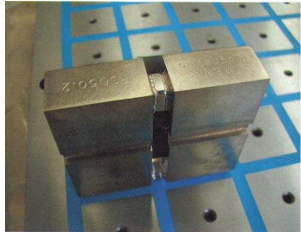
Transferring magnetism to side of part
